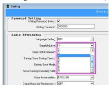
3)Relay Retransmission: Repeater automatic connect times. The number indicates the times radio automatic transmitting when not connect repeater successful after press PTT.
