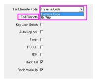
9)Key Lock Switch: Ticked and write it to the radio, when turn on the radio, the radio keypad is locked. You can long press "#" to unlock the keypad.
